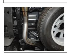
5. Install the Exit pipe onto the over axle pipe. Install hangers into the OEM rubber grommets. You may need to adjust each component to obtain optimal clearance. Use spacers if needed to lock parts in place while tightening down.
