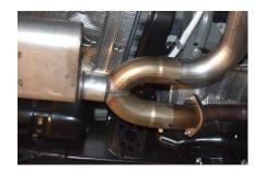
2. Install Item# A onto the factory Y-pipe re using the OEM Gaskets. Use the provide bolt kit Item G to secure the flanges to the factory pipes. Do not tighten.
