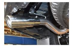
6. With proper clearance from spare tire install the exhaust tip onto the tailpipe. The system was designed to have the tip 1" below the quarter panel of the vehicle. With the tip in your desired position begin to tighten down all clamp connections from the front head pipe back.
