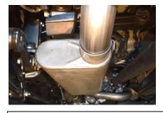
3. Install The Gibson Muffler Item #B onto the head pipe. The inlet will have the louvers facing forward. Look into the muffler to determine what direction is forward. The outlet will be clocked at the 3:00 position. Do not tighten
