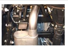
4. Install over axle pipe Item # C into the muffler outlet. Keep everything loose until the exit pipe is installed.
